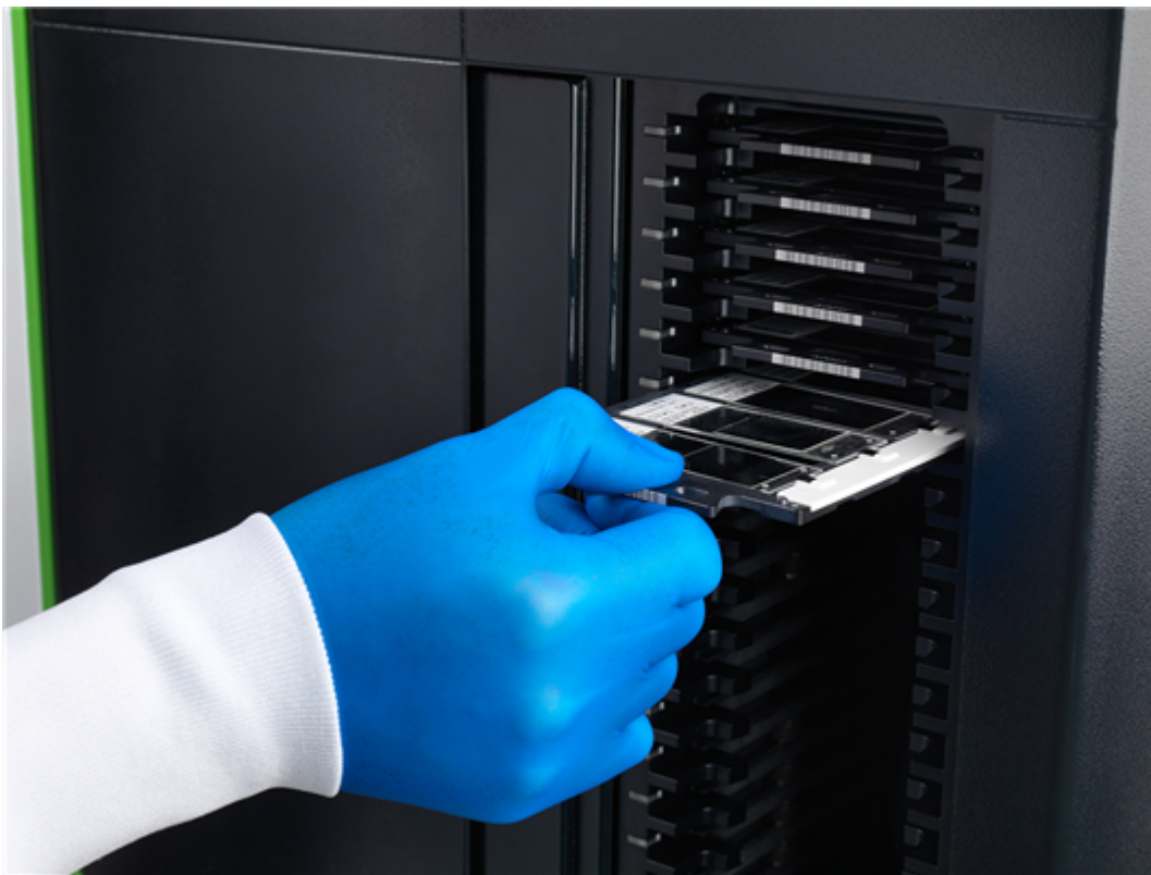
Figure 21. Push the Slide Carrier until Fully Seated
